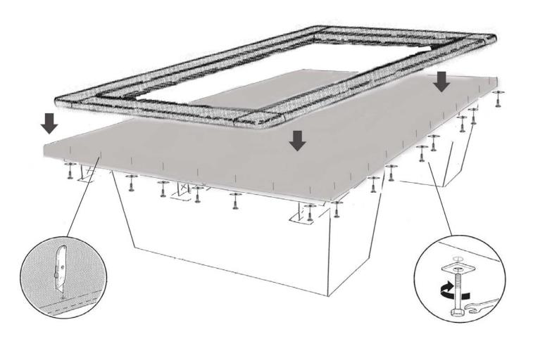
12. Last but not least — assemble the sides so they make a frame. Install the angle hinges to the sides with the screws. Finally put frame into the pre-drilled channel in the cushion-frame and fasten with the last 12 pcs. of loose BLACK bolts. Then fasten the bolts and your table is ready!
