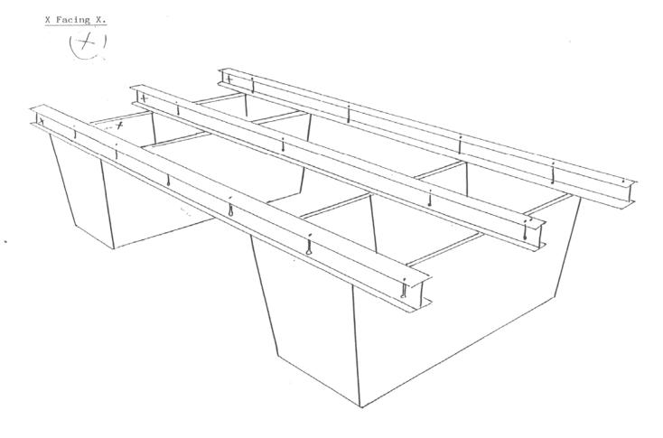
3. Place the bottom-frame on the steelbeams. The heatingsystem is integrated in the bottom-frame. Please test the function of the heating parts before continuing the setup of the table.
